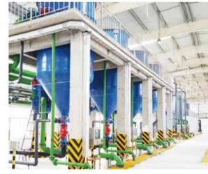
Membrane chemical reactor (MCR)
